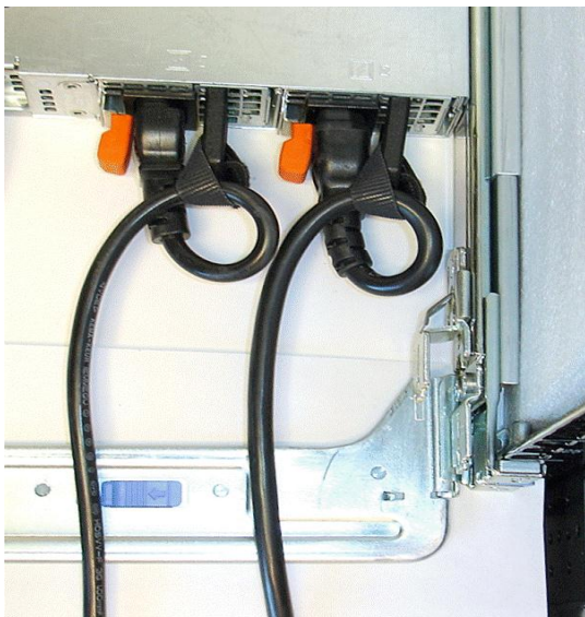
Figure 3: Routing Power Cables Through the Strain Reliefs
